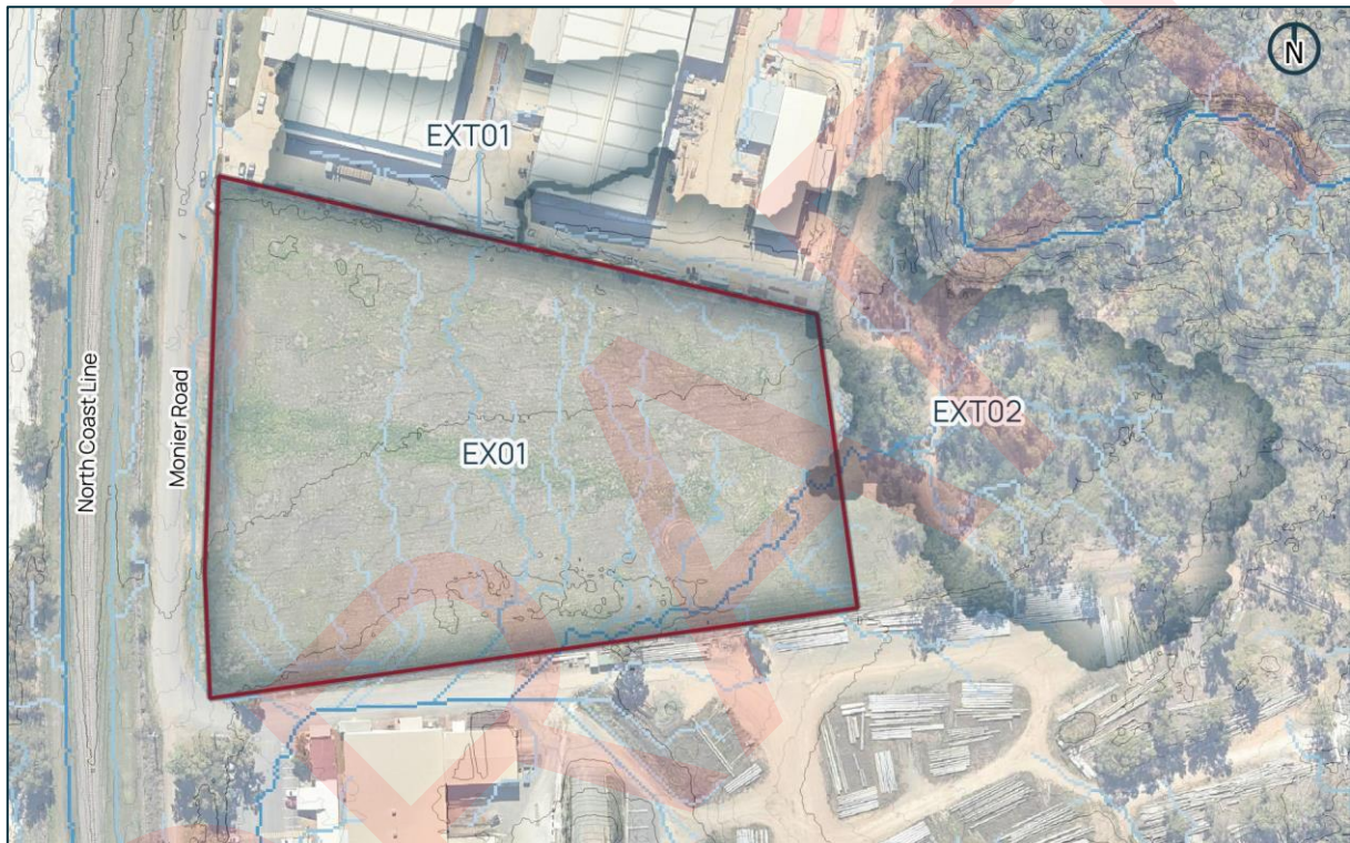
Figure 2 – Pre-development catchment layout plan
