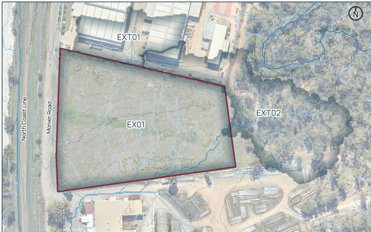
Figure 2 – Pre-development catchment layout plan
