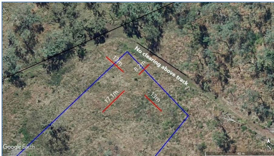
Figure 9. Minimum required APZ distances for each aspect around a dwelling. The distances are from the nearest facing surface of the dwelling to the hazard (woodland or unmanaged grass/shrubland). Additionally, the dwelling must not be in a location that would require clearing above the track shown in the image. There are a significant number of endangered cycads above the track.
