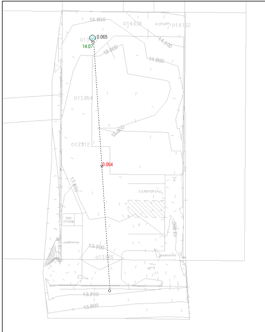
Figure 6 - Post-Developed Site Drains Model – No storage results
