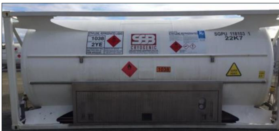
Figure 4 ISO Container – Side View Source: IXOM Operations Pty Ltd
