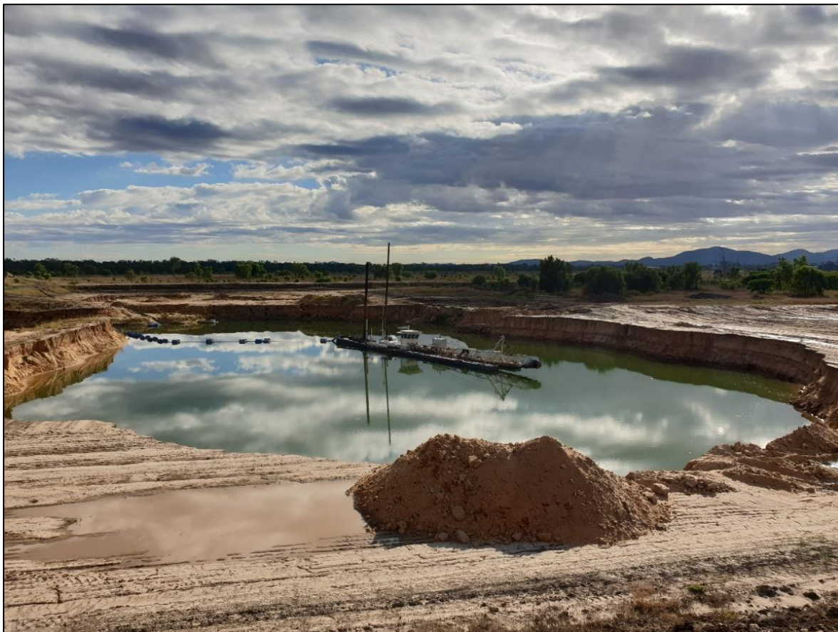
Figure 11. Floating dredge situated in extractive pit.
