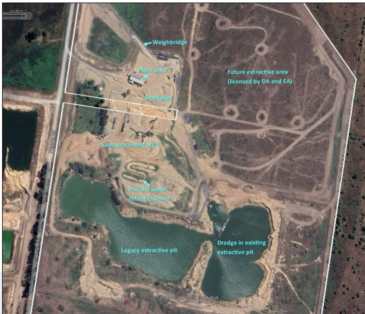
Figure 9. General layout of the extractive and screening activities. Note the sediment collection/water return channel which captures fine sand and sediment prior to it entering the main retention basin. [Source: Google Earth, imagery date October 2022].
