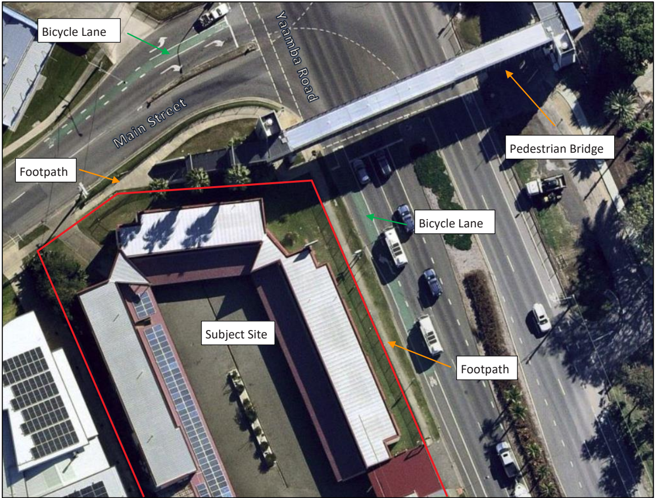
Figure 2.8: Pedestrian and cyclist infrastructure in the vicinity of subject site [Source: Nearmap]
