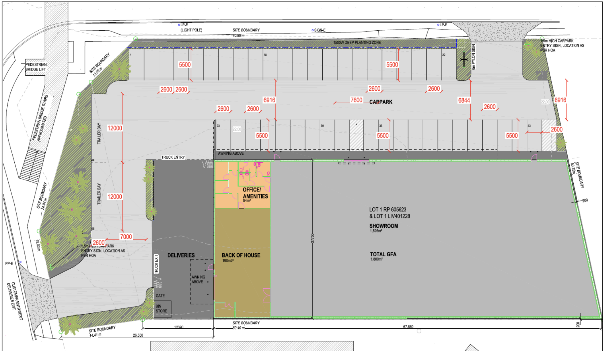
Figure 4.1: Dimensioned car parking layout
