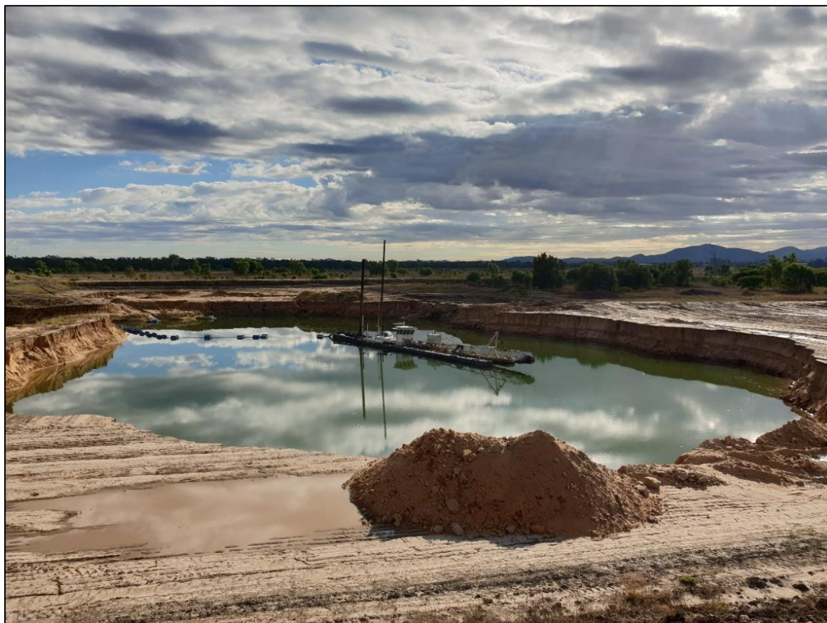
Figure 11. Floating dredge situated in extractive pit.
