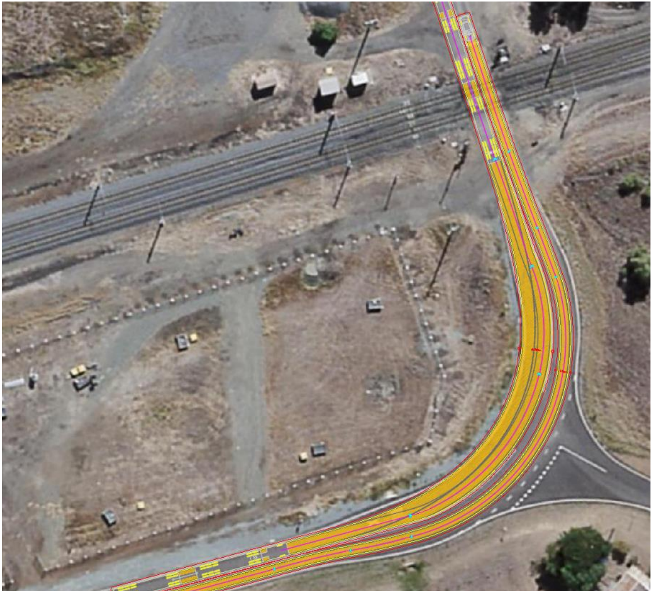
Figure 10-12: A-Double travelling northbound (Second Street / Riverslea Road corner)
