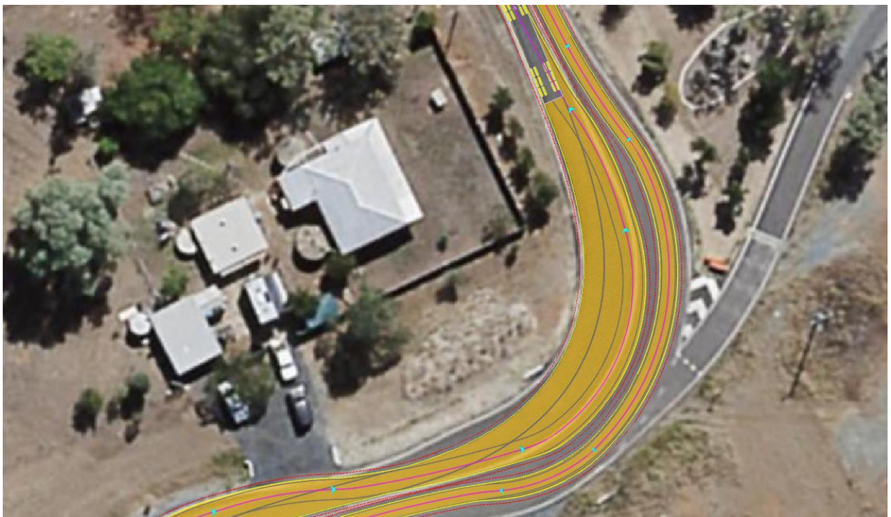
Figure 10-4: A-double travelling northbound along Third Street – crossing centre line
