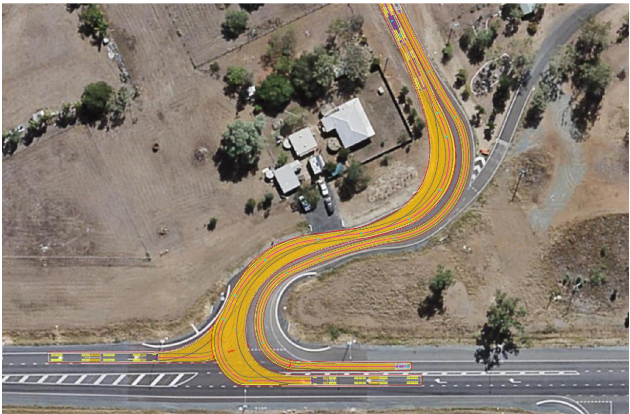
Figure 10-2: A-double travelling northbound along Third Street (without crossing centre line)
