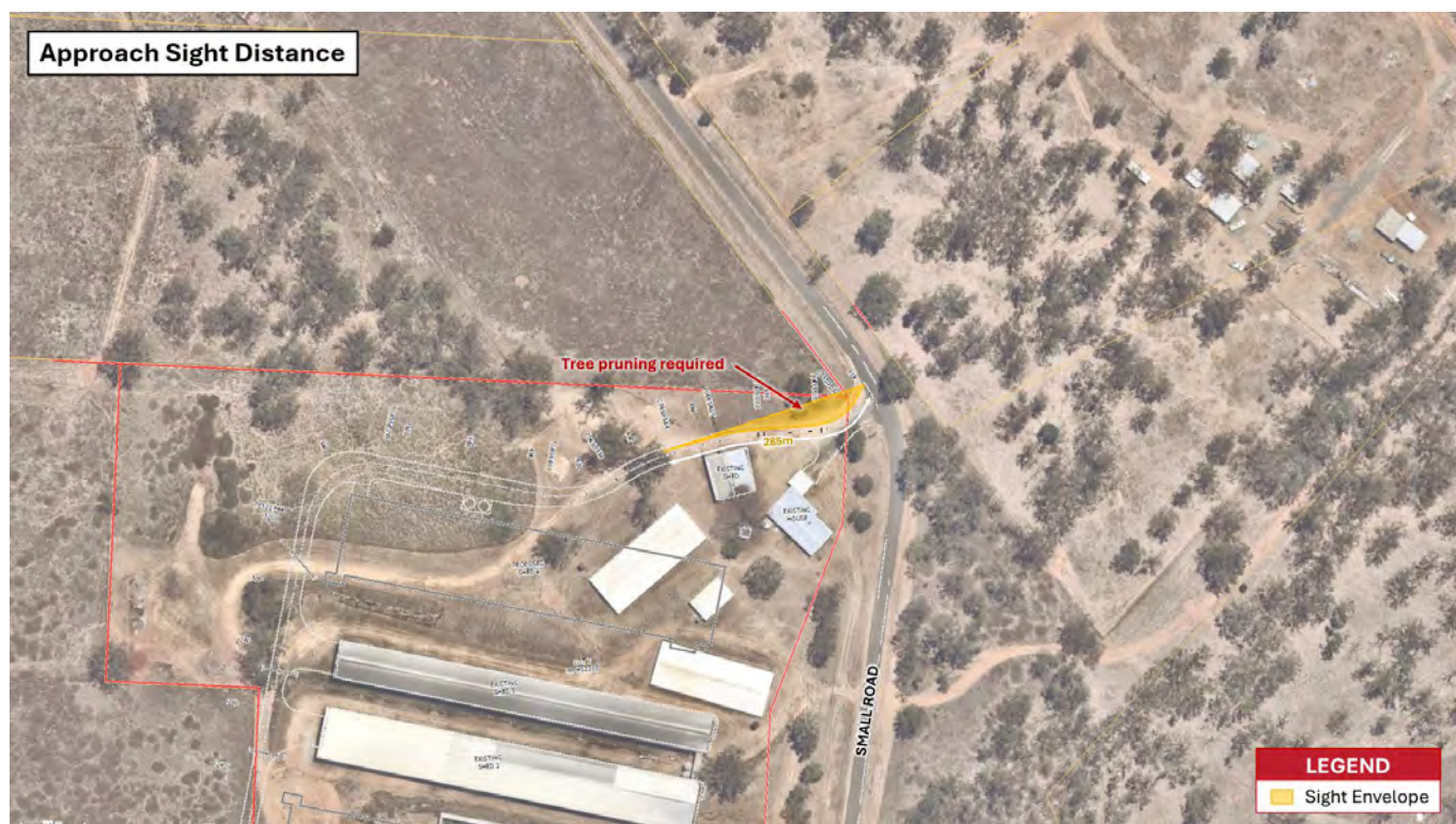
Figure 1: Approach Sight Distance (Source: Nearmap, PSA)
