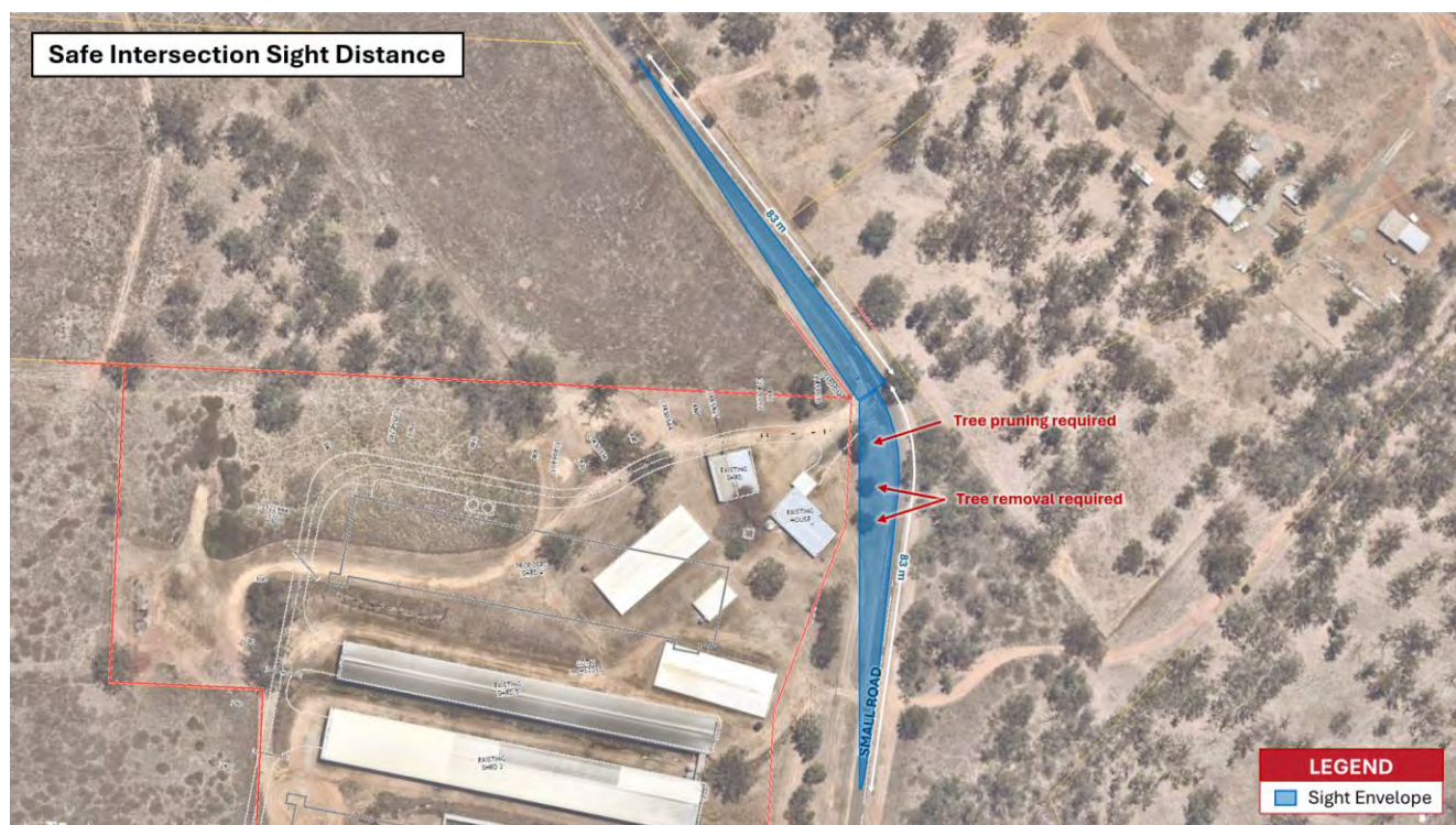
Figure 3: Safe Intersection Sight Distance (Source: Nearmap, PSA)
