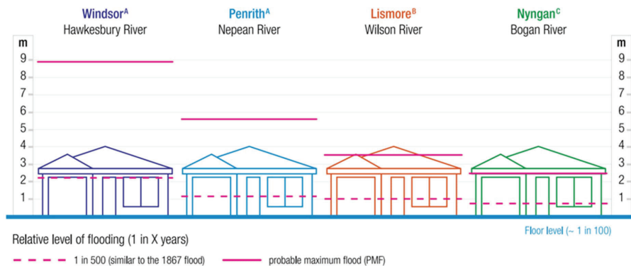
Figure E7 Example of a Comparison of Differences in Flood Levels and Residual Risk (INSW, 2017)
